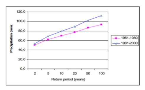
Figure 5 - Comparison of 24-Hour Precipitation Between 1961-1980 and 1981-2000 at Station G6140954
