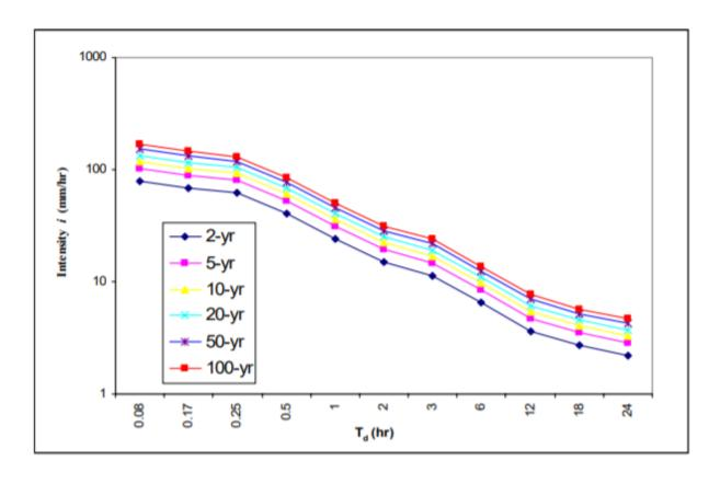
Figure A10 – IDF Curves for Observed Precipitation (1981-2000) at Station G6140954
