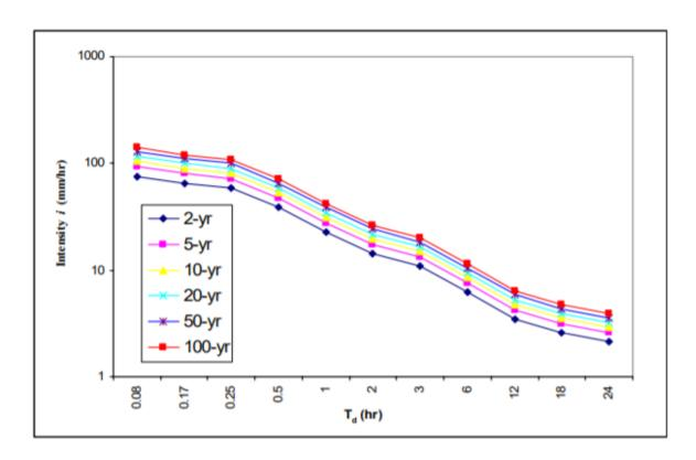
Figure A9 – IDF Curves for Observed Precipitation (1961-1980) at Station G6140954
